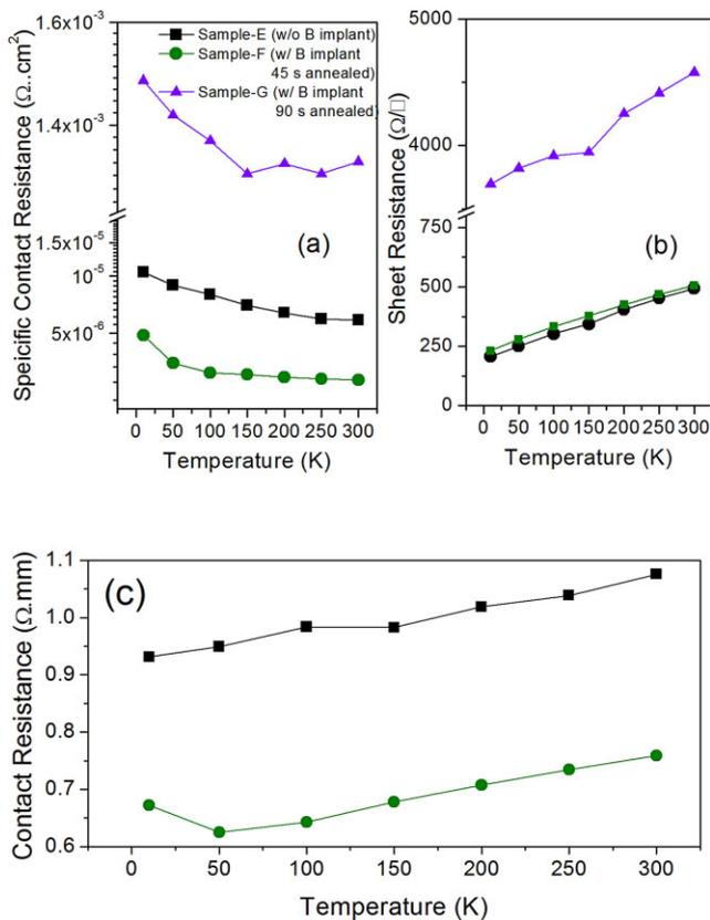
**Figure 6** (a) Specific contact resistance, (b) sheet resistance, and (c) contact resistance as a function of temperature for as-grown and B implanted AlGaN/GaN heterostructures. The specific contact resistance reduces due to trap assisted tunneling. The B impurities in the channel region critically reduce the 2DEG conductance. The sheet resistance increases with temperature due to increased phonon scattering and reduced mobility.
