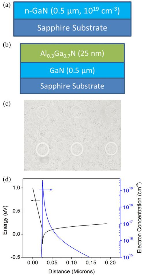
**Figure 1** Schematic of (a) Si-doped bulk GaN and (b) AlGaN/GaN heterostructure for HEMT devices; (c) micro-photograph of the fabricated CTLM geometry. (d) Simulated band diagram and electron density plot showing that a two-dimensional electron gas (2DEG) is formed at the AlGaN/GaN interface. Efficient tunneling between the contact and 2DEG is a pre-requisite for low resistance Ohmic behavior.
