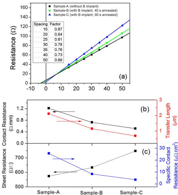
**Figure 4** (a) Resistance versus separation for as-grown and B implanted (annealed for 45 s and 90 s) samples. The resistance decreases for B implanted samples. (b) Contact resistance and transfer length, (c) sheet resistance and specific contact resistance plotted for as-grown and B implanted samples. The specific contact resistance decreases, however, sheet resistance increases due to B implant.
