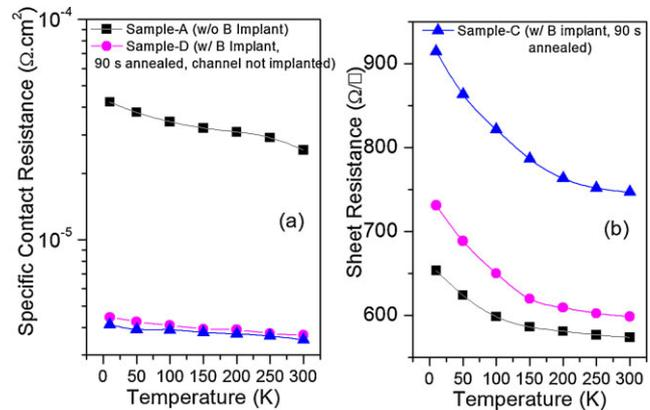
**Figure 5** (a) Specific contact resistance and (b) sheet resistance as a function of temperature for as-grown and B implanted samples. The specific contact resistance for B implanted sample is relatively independent of temperature as tunneling is the dominant mechanism for electron transport. Sheet resistance reduces with increasing temperature due to increased ionization of Si dopants at higher temperature.
