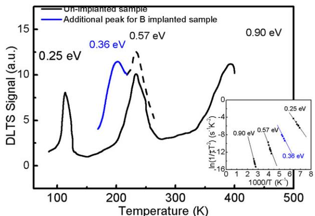
**Figure 7** DLTS characteristics for un-implanted and B implanted samples. B gives rise to a new trap level at 0.36 eV below the conduction band edge. The Arrhenius plot is shown in the inset.
