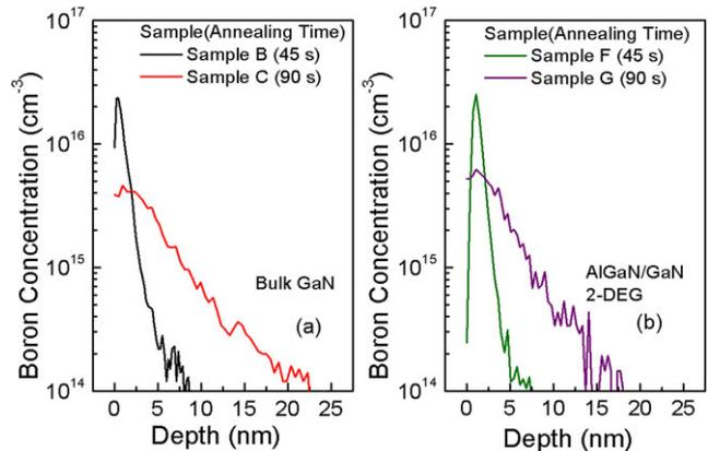
**Figure 2** Boron depth profile for 45 s and 90 s annealed (a) bulk GaN and (b) AlGaN/GaN heterostructure samples. The penetration depth increases with increasing annealing time. A total of 90 s annealing leads to B very near to the two-dimensional electron gas in sample G leading to degraded sheet resistance.
